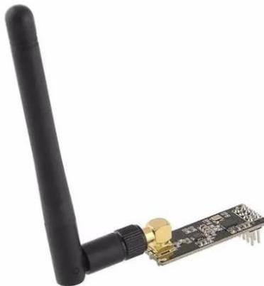
Figura 32. Antena NRF24I01[14]
