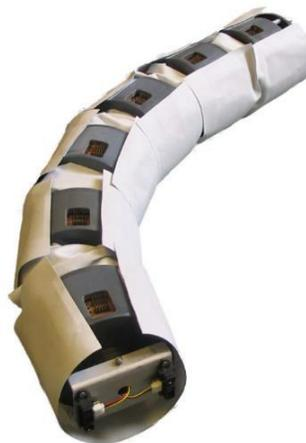
*Figura 4. The Pneumosnake robot [10].*
