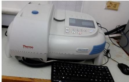
**Figura 3. Thermo Scientific Evolution 201 UV-Visible Spectrophotometer.**
