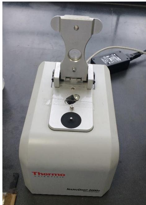
**Figura 4. Thermo Scientific NanoDrop® 2000C Spectrophotometer.**
